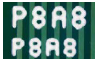
NEW: 0.7 & 0.6 mm text with DotStream Pro technology one pass, 15 sec** (Orbotech Sprint 200)
