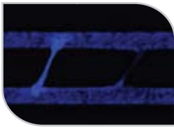
Blue light image - clear distinction between dust and fine short (dust is much brighter)
